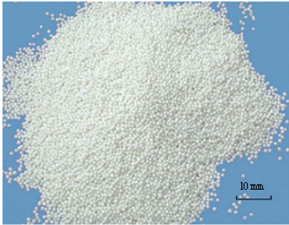
Fig. 20. ZrO_2 microbeads of ceramics prepared by gel-bead forming technique.
